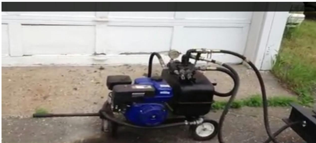
Fig No.4 Assembled Hydraulic Power Pack
